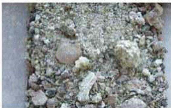
Fouling glass furnace
